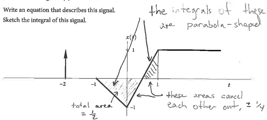
(a)  $\delta(t+2) - \text{ramp}(t+1) + 3 \cdot \text{ramp}(t) - 2 \text{ramp}(t-1)$
