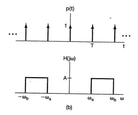
To examine the possibility of sampling a bandpass signal as a rate less than the total bandwidth, consider the system shown in Figure P7.26(b). Assuming that  $\omega_1 > \omega_2 - \omega_1$ , find the maximum value of T and the values of the constants A,  $\omega_a$ , and  $\omega_b$  such that  $x_r(t) = x(t)$ .
