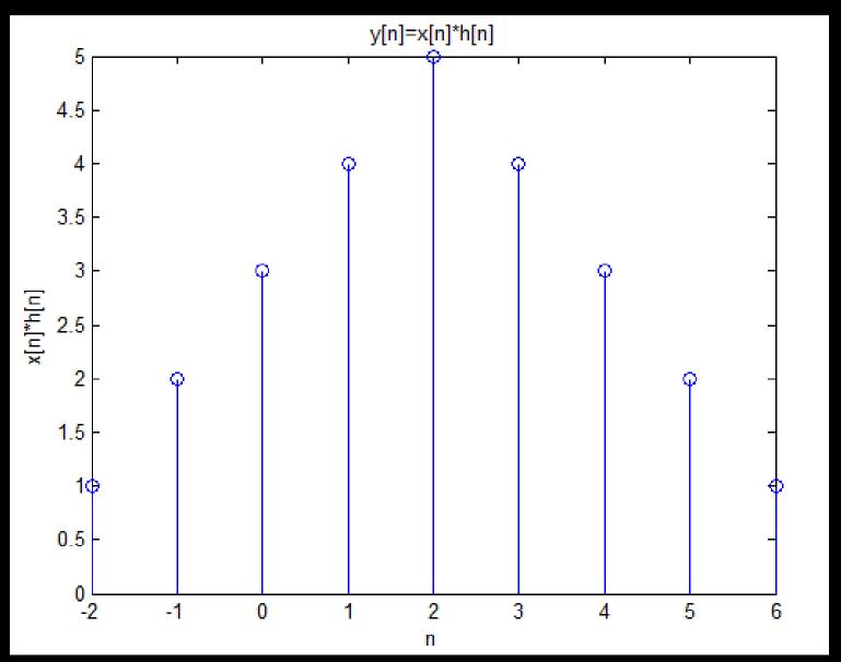
$\therefore y[n] = \delta[n+2] + 2\delta[n+1] + 3\delta[n] + 4\delta[n-1] + 5\delta[n-2] + 4\delta[n-3] + 3\delta[n-4] + 2\delta[n-5] + \delta[n-6]$
