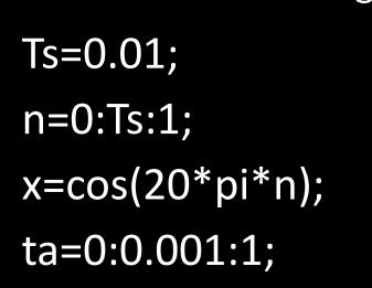
Spline Code %time window %time index %sampled signal %reconstruction time
