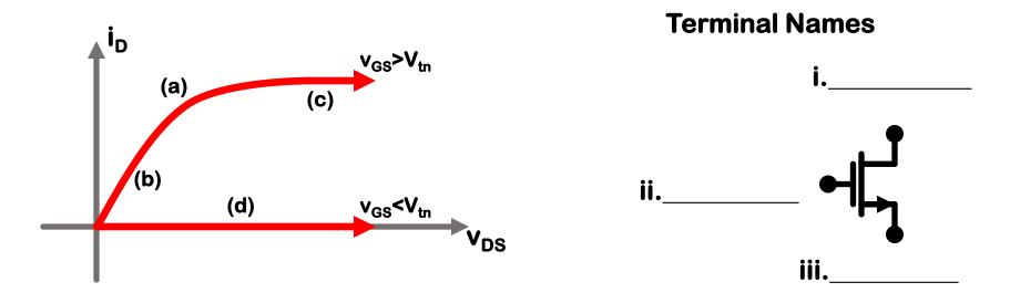
Channel Shapes (No Channel, Rectangular, Tapered, Triangular)
