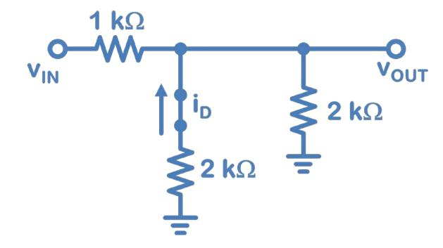
Find  $v_{OUT}(v_{IN})$  and the range of  $v_{IN}$  that Reverse Bias is valid.
