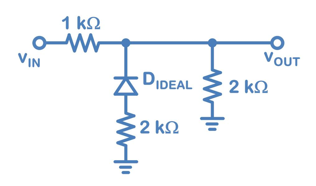
Find  $v_{OUT}(v_{IN})$  and the range of  $v_{IN}$ . Do both FB and RB.
