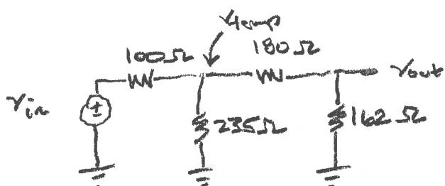
$$\frac{v_{temp}}{v_{in}} = \frac{1.39}{100 + 1.39} = 0.58$$
