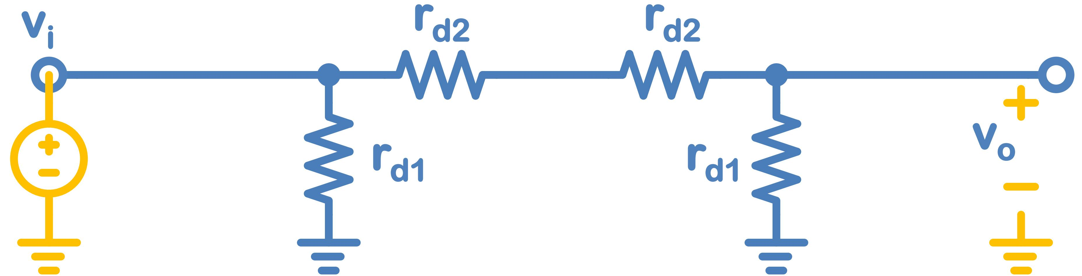
$$v_o/v_i = r_{d1}/(2r_{d2} + r_{d1})$$
