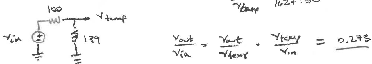
$$\frac{v_{out}}{v_{in}} = \frac{v_{out}}{v_{temp}} \cdot \frac{v_{temp}}{v_{in}} = 0.273$$
