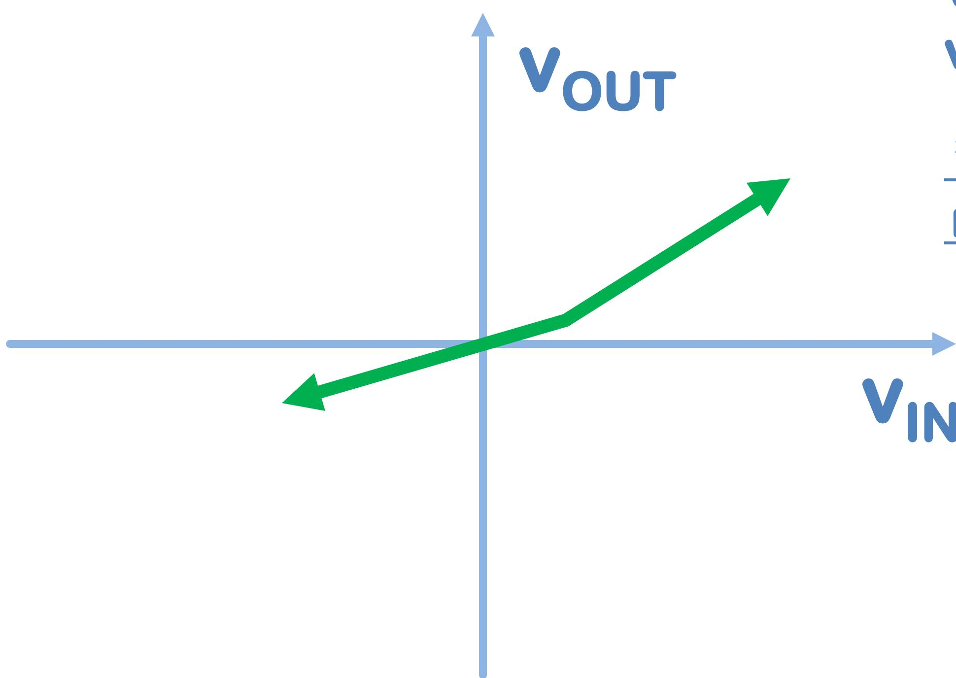
$$v_{OUT} = (1/3)v_{IN}, \text{ when } v_{IN} < 3.15$$
