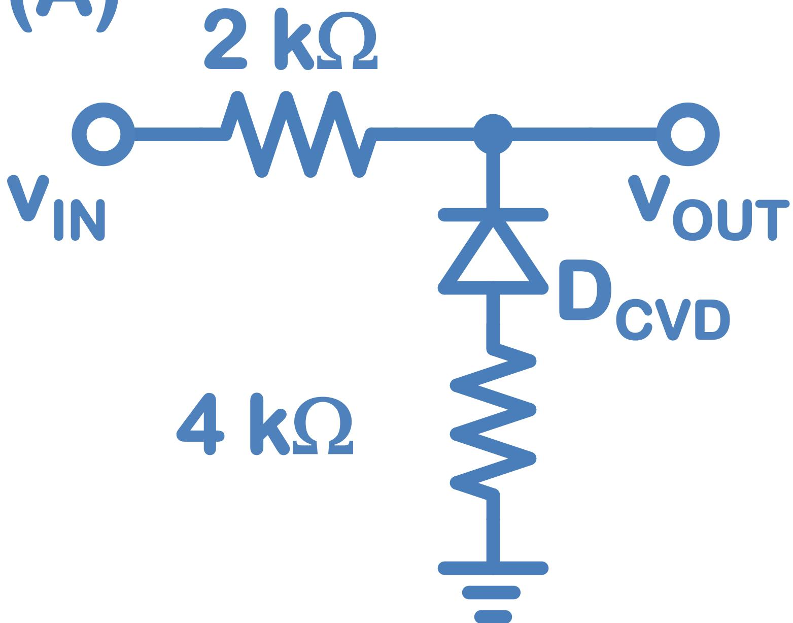
$$v_{OUT} = .67v_{IN}, -.23 \text{ when } v_{IN} < -0.7$$
