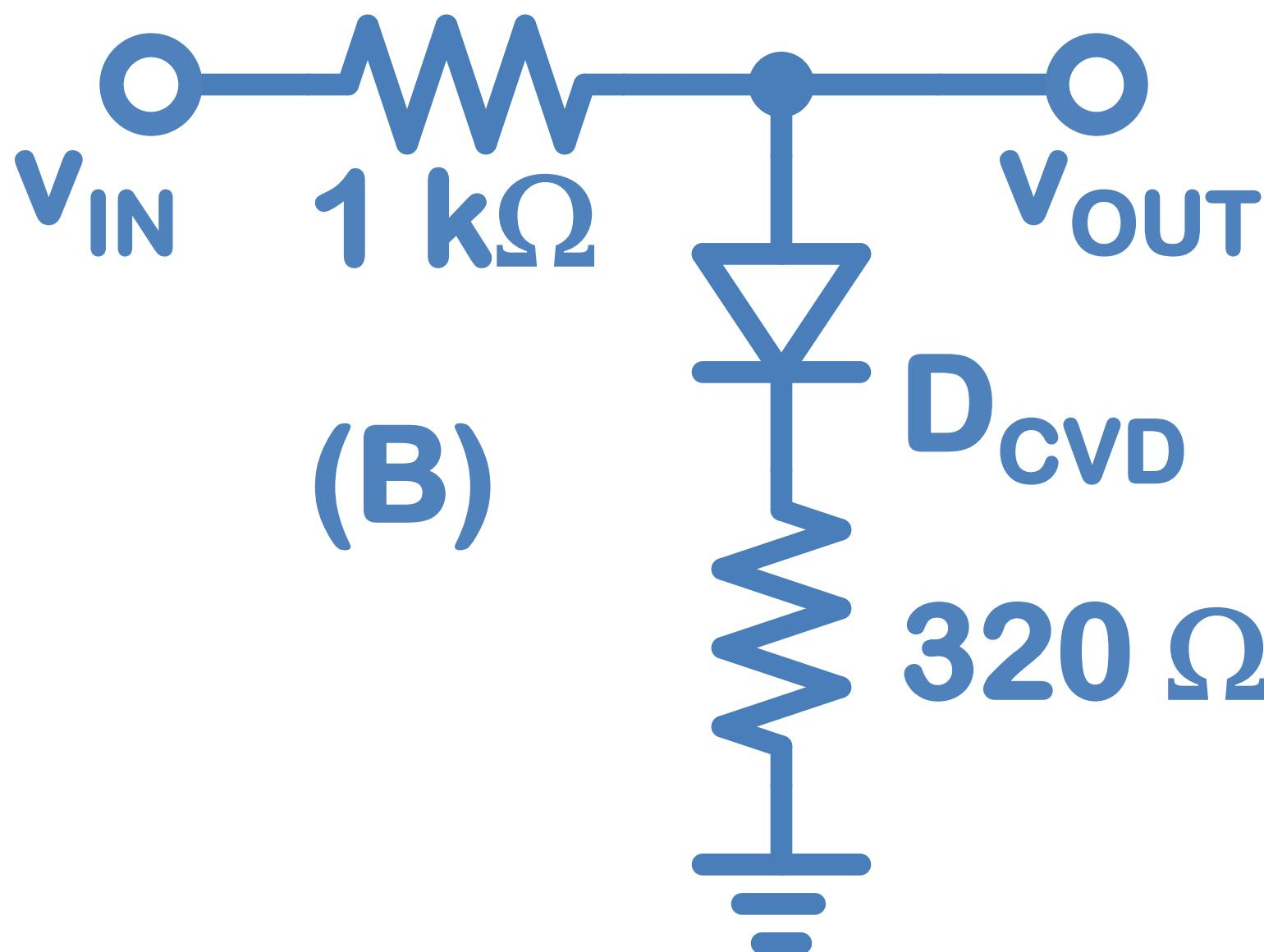
$$v_{OUT} = v_{IN}, \text{ when } v_{IN} < 0.7$$
