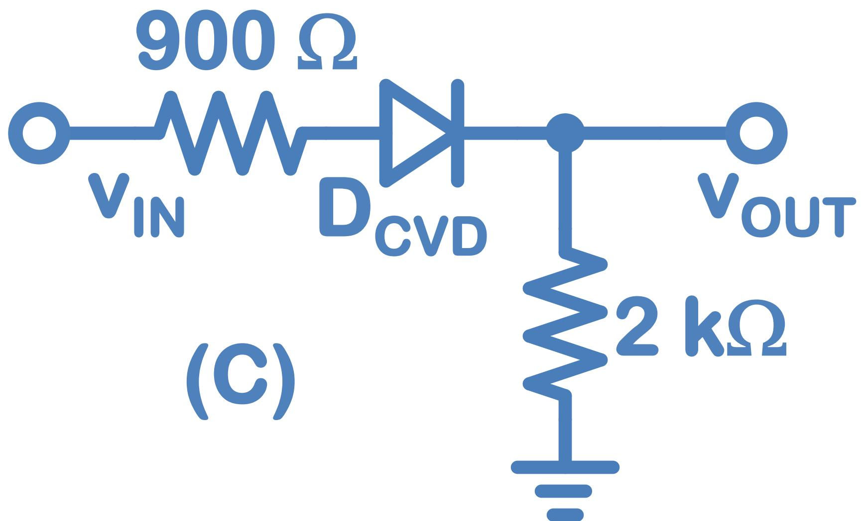
$$v_{OUT} = 0.7(v_{IN} - 0.7) \text{ when } v_{IN} > 0.7$$
