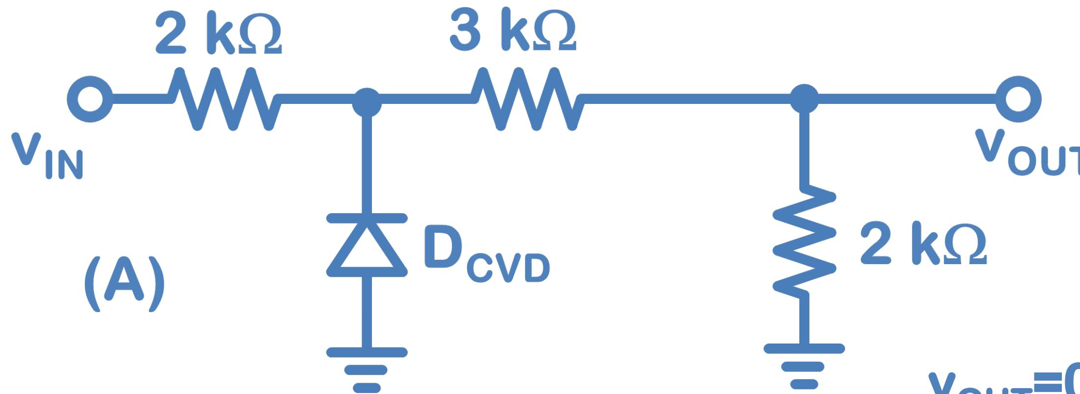
$$v_{OUT} = 0.28, \text{ when } v_{IN} < -0.98$$
