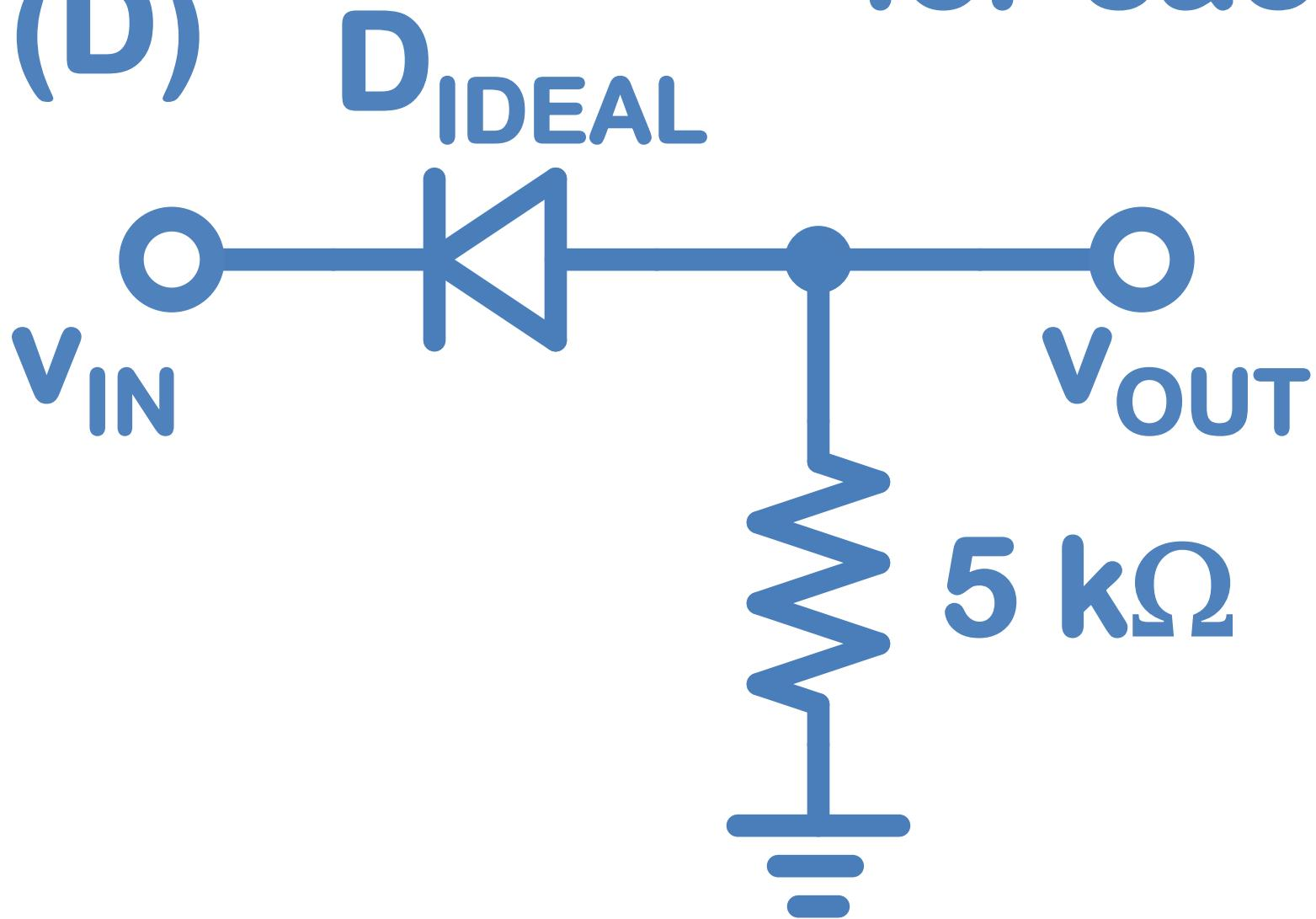
$$v_{OUT} = 0, \text{ when } v_{IN} > -0.7$$
