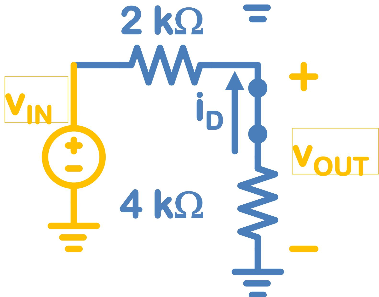
$$v_{\text{OUT}} = 0.67v_{\text{IN}}$$
