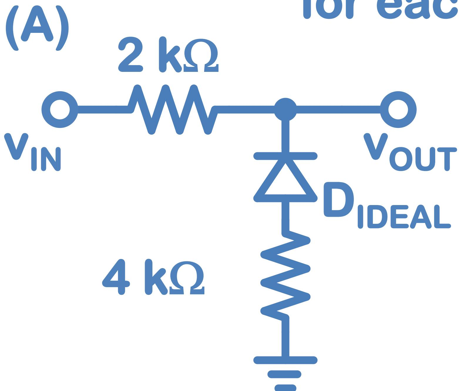
$$v_{OUT} = .67v_{IN}, \text{ when } v_{IN} < 0$$
