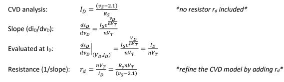
Values of  $R_s = 1 \text{ k}\Omega$ , n = 2, and  $v_s = 3.5 \text{ V}$  results in  $r_d = 35.7 \Omega$  and a line regulation of  $\Delta v_R / \Delta v_s = 0.096$ .
