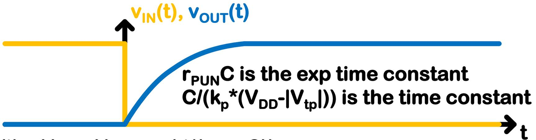
$$v_{OUT}(t) = V_{DD} - V_{DD} \cdot \exp(-t/(r_{PUN} \cdot C))$$
