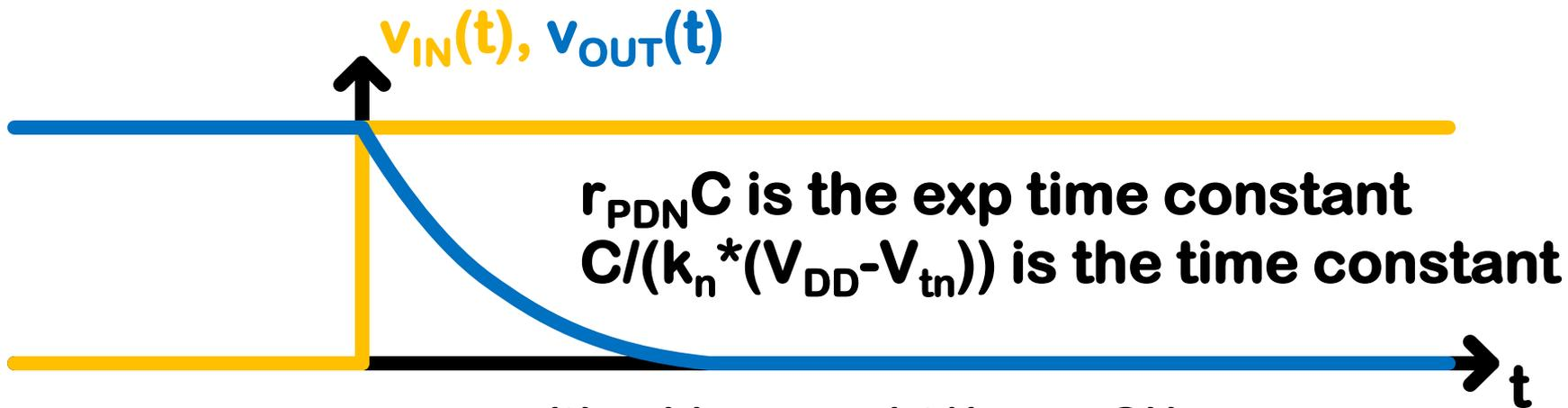
$$v_{OUT}(t) = V_{DD} \cdot \exp(-t/(r_{P_{DN}} \cdot C))$$
