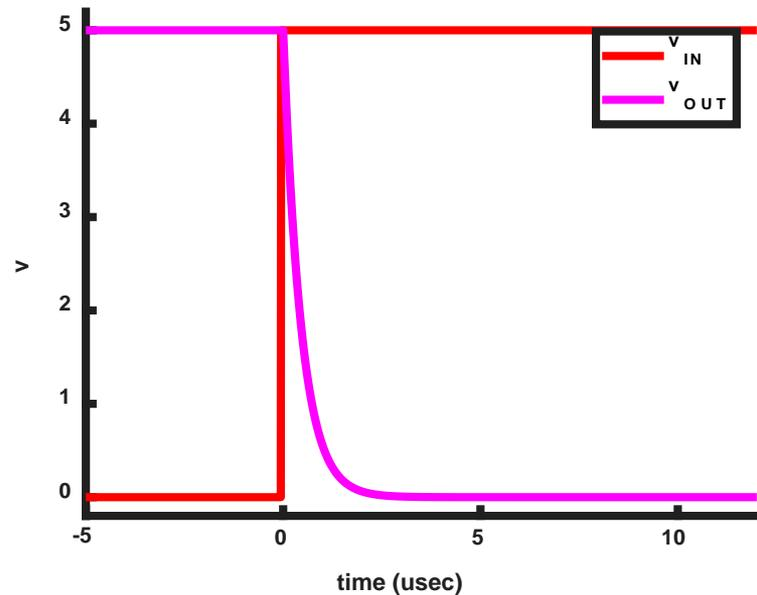
$$v_{OUT}(t) = V_{DD} \cdot \exp(-t/(r_{PDN} \cdot C))$$
