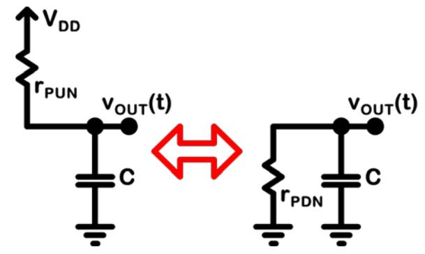
$$P_{SUPPLY} = (V_{DD}^2/r_{PUN}) \cdot \exp(-t/(r_{PUN} \cdot C))$$
