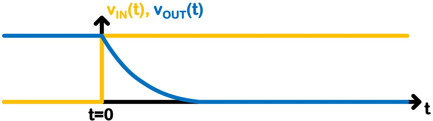
$$v_{OUT}(t_{50}) = V_{DD} \cdot \exp(-t_{50}/(r_{PDN} \cdot C)) = V_{DD}/2$$
