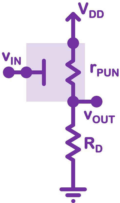
$$r_{PUN} = r_{SD} = 1/(k_p(v_{DD} - |V_{tp}|))$$
