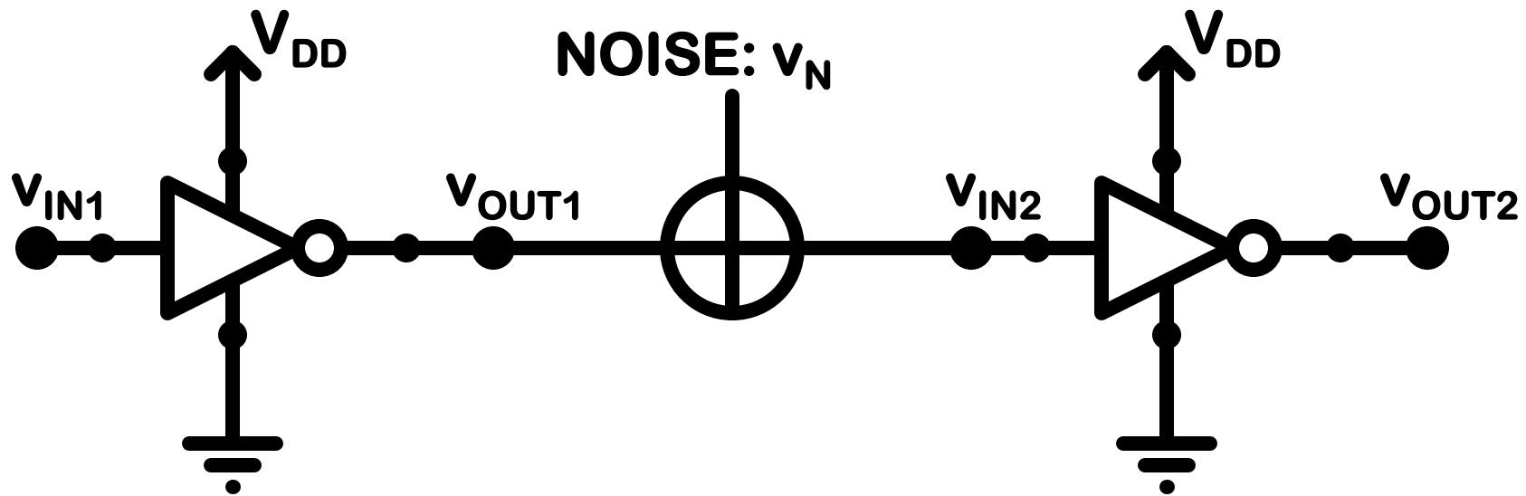
**NOISE MARGIN:** The maximum magnitude of noise that the circuit can tolerate to ensure  $v_{IN2}$  stays out of the transition region.
