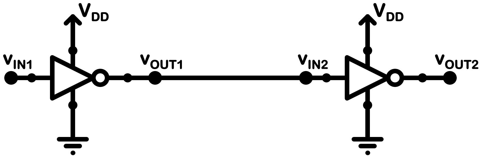
As long as the input is at least 2.0V, the input is registered high and the output will be low with a voltage that is at most 0.4V. ( $v_{IN} > 2.0$ ,  $v_{OUT} < 0.4$ )
