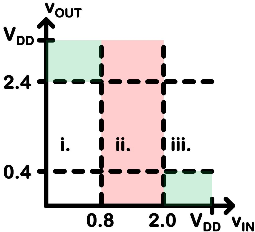
As long as the input is at least 2.0V, the input is registered high and the output will be low with a voltage that is at most 0.4V. ( $v_{IN} > 2.0$ ,  $v_{OUT} < 0.4$ )
