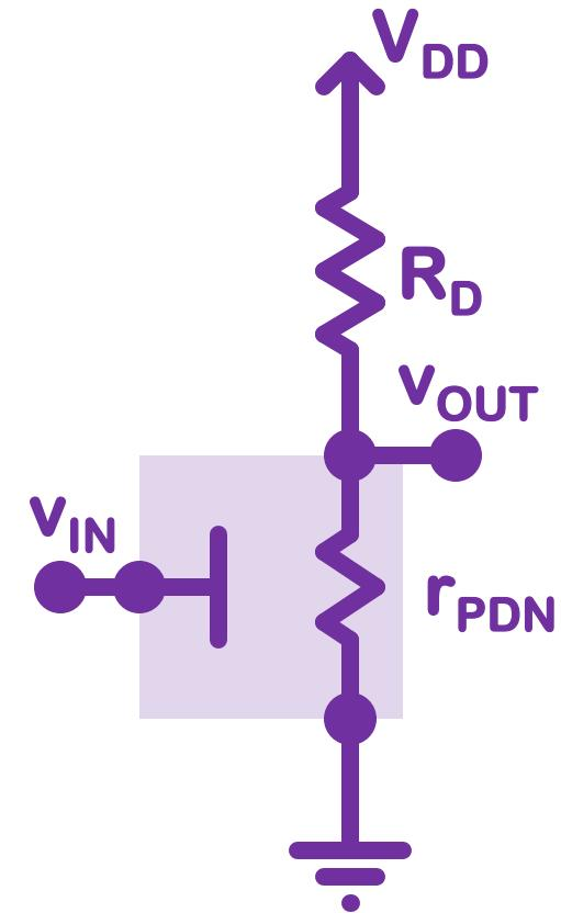
$$r_{PDN} = r_{DS} = 1/(k_n(v_{DD}-V_{tn}))$$
