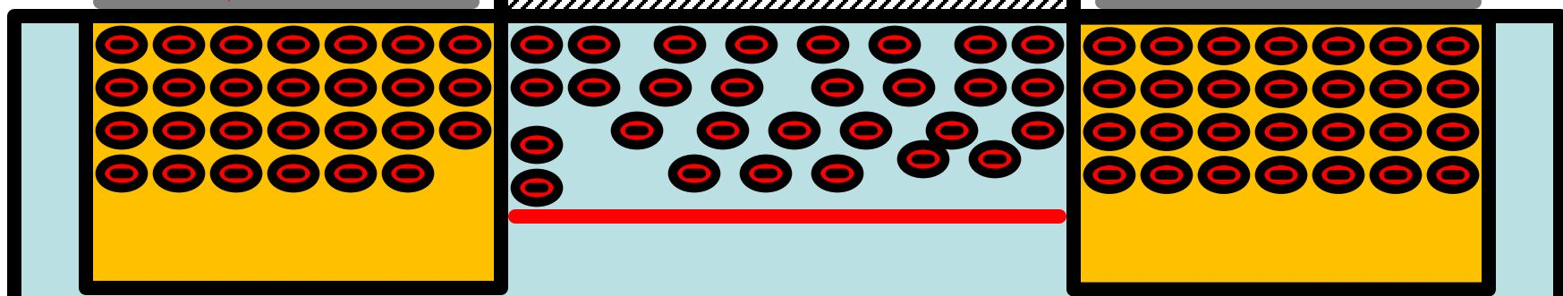
$$r_{DS} = L / [\mu_n \cdot C_{ox} \cdot W \cdot (v_{GS} - V_t)]$$
