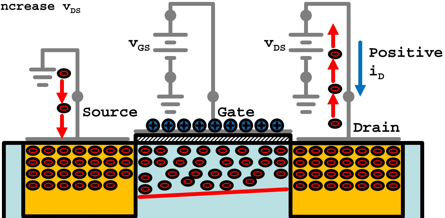
$$r_{DS} = L / [\mu_n \cdot C_{ox} \cdot W \cdot (v_{GS} - V_t)]$$
