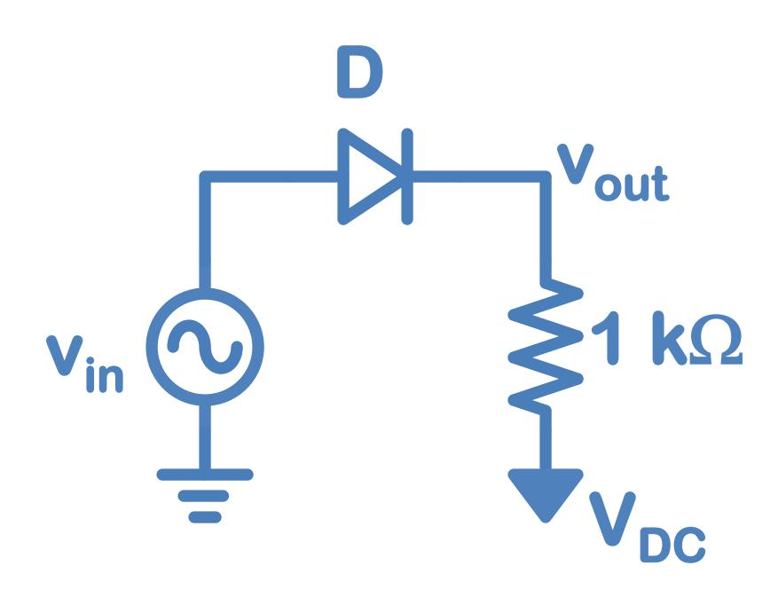
A large signal current is generated through the diode to set the small signal resistance.
