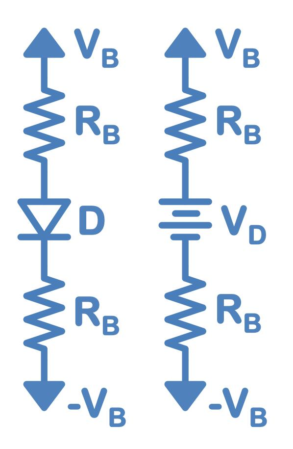
$I_{\rm D} = (2V_{\rm B} - V_{\rm D}) / (2R_{\rm B})$  $V_{\rm D} = 2V_{\rm B} - 2R_{\rm B}I_{\rm D}$ For a typical junction diode,  $I_D$ can span several orders of mangnitude (0.1mA to 100mA) for small changes (deltas) in V<sub>D</sub> (+/-100mV) around 0.7V.
