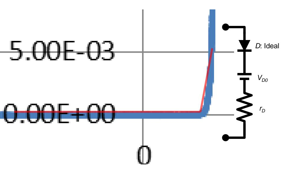
$V_{D0}$ =0.6 V and  $r_{D}$ =20  $\Omega$ .
