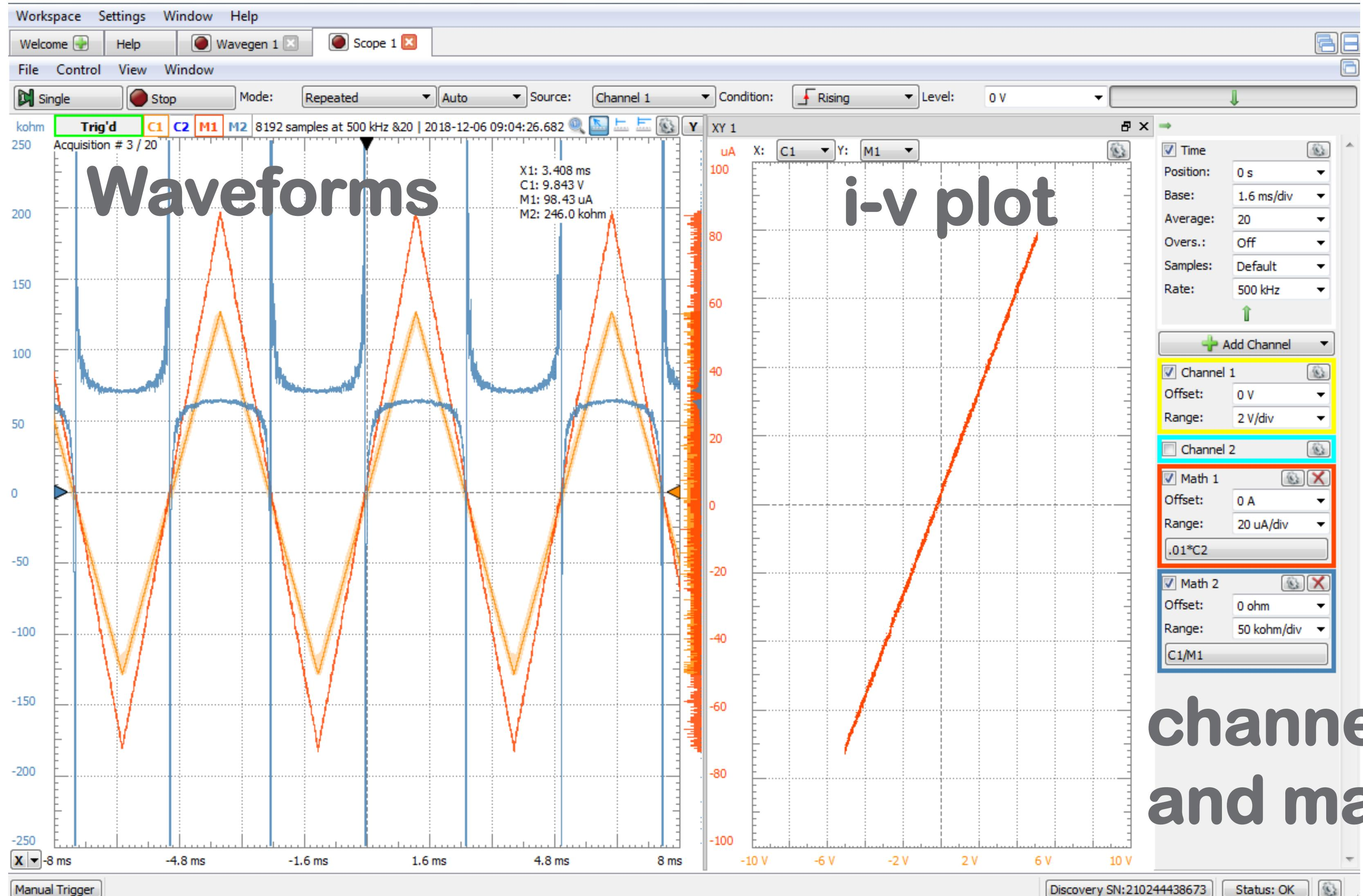
$$R = v_R/i_R = 1/(i-v \text{ slope}) = 100 * (\Delta C_1)/(\Delta C_2)$$
