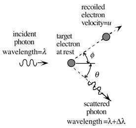
In this experiment, photons of wavelength  $\lambda$  bombard an electron initially at rest. After the collision, the electron would recoil at some angle  $\phi$  and a new, downshifted, photon would be emitted at an angle  $\theta$ . Equating the electron+photon energy and momentum before and after the collision, the following relationship can be derived between the wavelength shift  $\Delta\lambda$  and the angle shift  $\theta$  of the photon:
