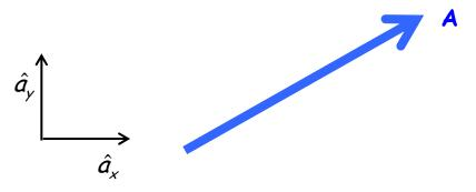
By using the **dot product**, we find the component of vector **A** in the direction of basis vector  $\hat{a}_x$ .
