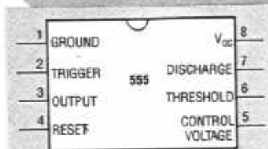
FIG. 1—PINOUT DIAGRAM OF THE 555.
