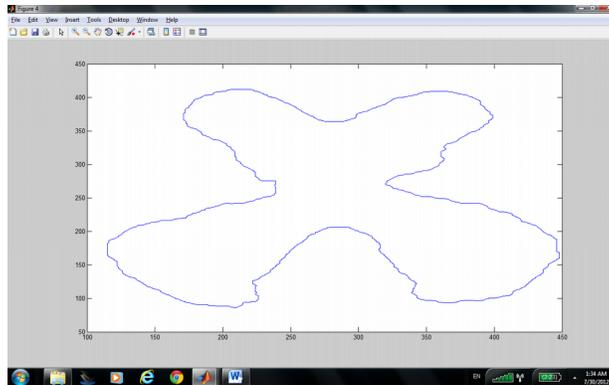
And then, with the boundary contour, we have to generate the mesh file. To do that, run `post_process_contour.m`.
