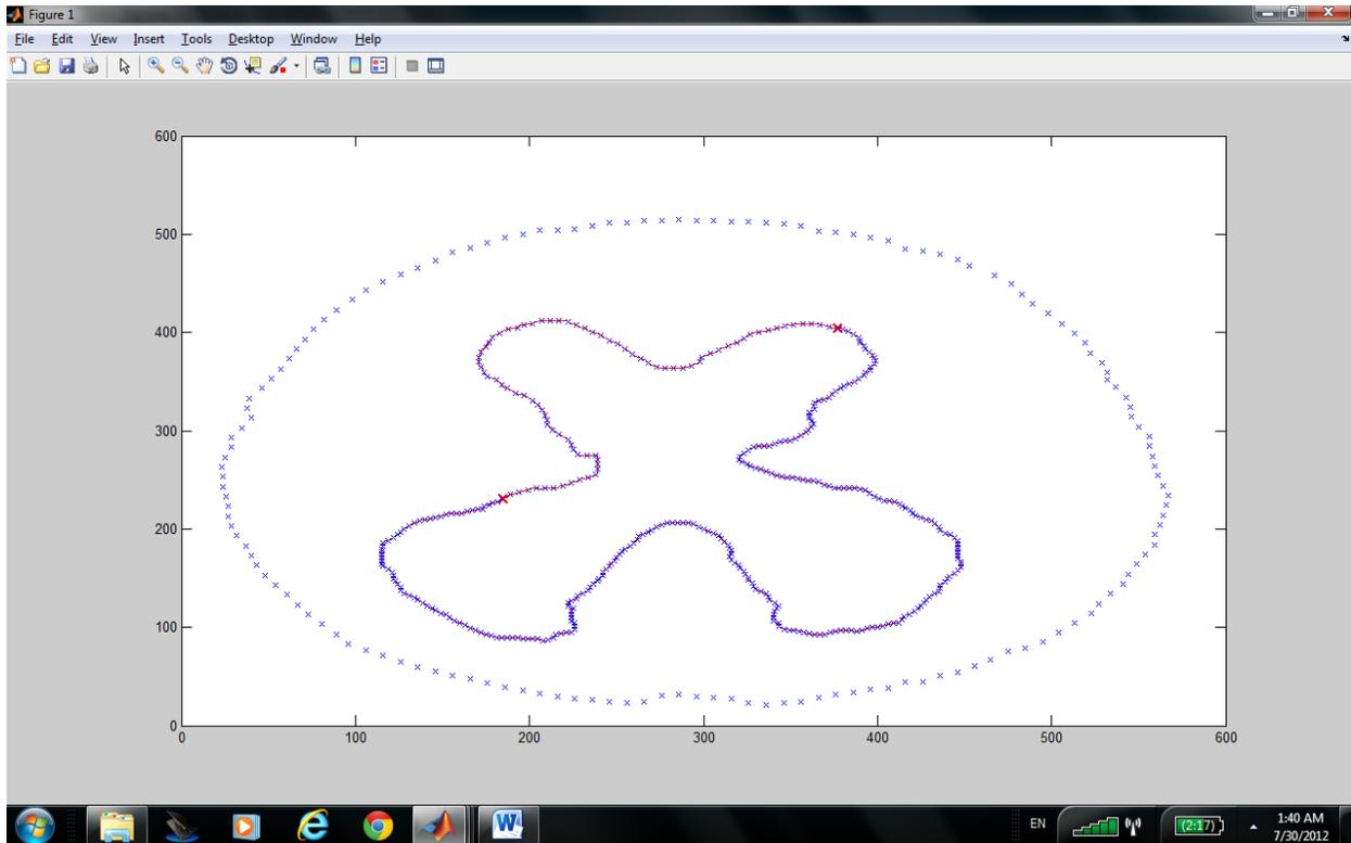
The poly file is named “init\_to\_inter\_lsm\_10\_boundary.poly” and stored. By using this file as a target mesh boundary, mesh warping process with FEMWARP will be processed.
