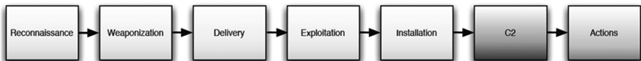
Fig. 3. The Lockheed-Martin Killchain Eric Hutchins and Amin (2011) depicts a seven phase attack lifecycle.
