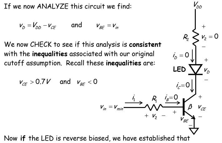
Now **if** the LED is reverse biased, we have established that  $v_D < 0.5 V$ , meaning that for this circuit assumption
