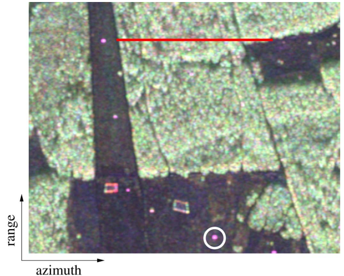
Fig. 9. Full polarimetric SAR composite master image with R(HH)–G(HV)–B(VV) color coding. The forested area is analyzed along the cut represented by the straight line. The point identified by the circle represents two corner reflectors in a layover geometry.
